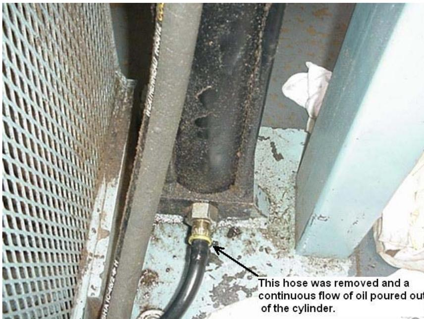
It was also mentioned that the previous week the stacker had *not* been drifting down with the locking valve solenoid de-energized. This would indicate a problem with the Moog valve or bypassing in the manifold.
