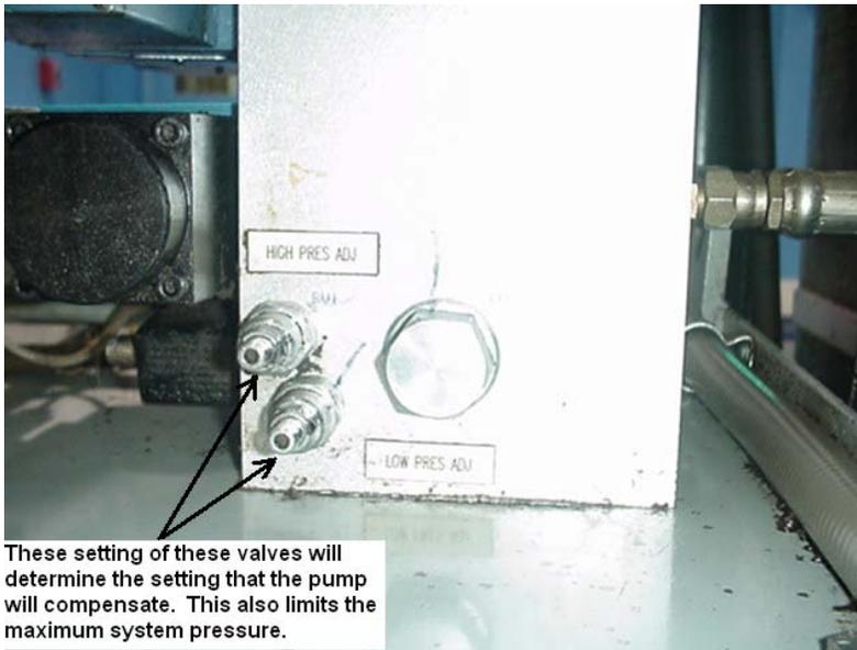
It was also mentioned that the drifting stopped when the high pressure setting was selected. Since the low pressure setting is not high enough to hold the stacker up, the oil could be flowing through the "P" port of the Moog valve and bleeding down through the pump. The check valve CXHA-LCN would have to be stuck open for this to occur. This check valve can
