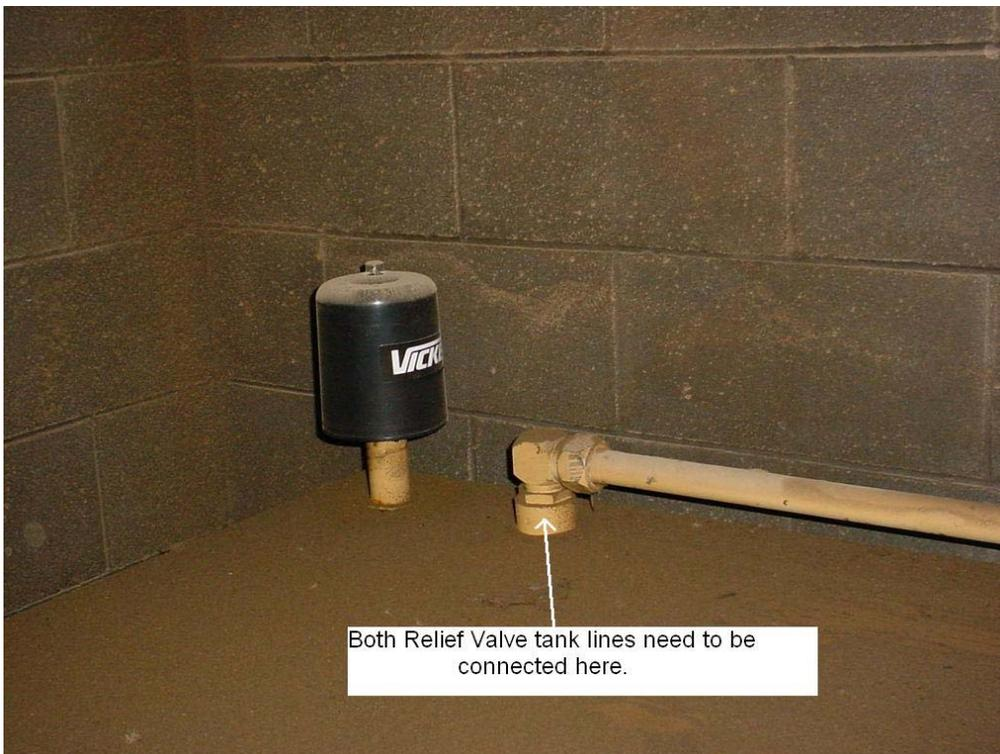
I also recommend to use the vickers high flow relief valve, 3000 PSI max pressure.
