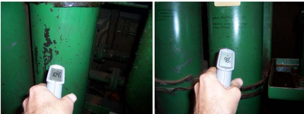
If the shell is cool all over then the accumulator is over-charged, oil is on top of the piston or all the nitrogen has leaked out. If it is hot all the way to the top, the pre-charge is too low.
